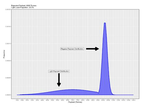
For Model implementation, a test is performed every time a train presents at a TLO to determine whether the Payload will be a light load or a full load. The Payload is then sampled from the corresponding distribution.
