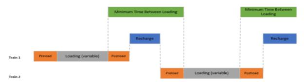
At terminals with multiple Inloaders, loaded trains arriving at the terminal are placed in a queue awaiting an available Inloader. Loaded trains are only allocated to an available Inloader when the next one becomes available. Inloaders serve trains on a first-come first-served basis.
