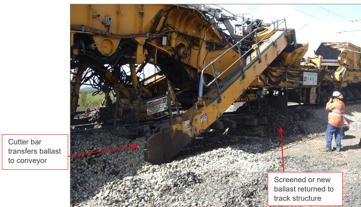
Figure 2 – RM900 cutter bar area
