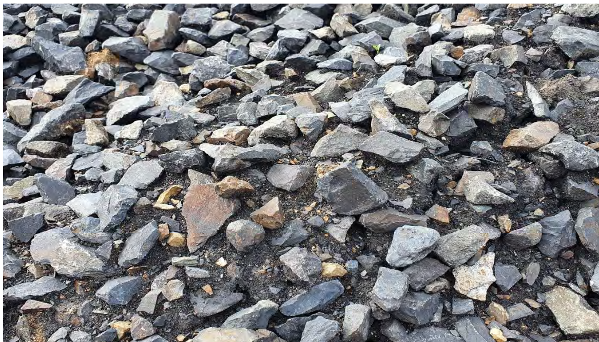
Figure 5-1 Stockpiled removed ballast
