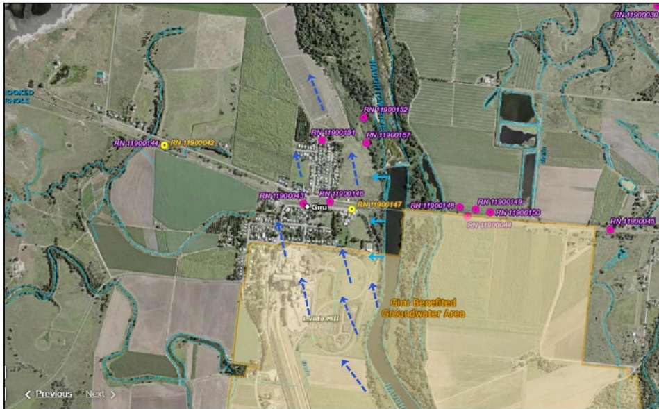
Figure 10 - Location of DNRME Bore 11900147. The royal blue arrows indicate the flow direction of groundwater, in old river channels (part of the aquifer), which leaves the area towards the North. Pale blue arrows indicate the continuous flow of surface water into the aquifer from the weir.
