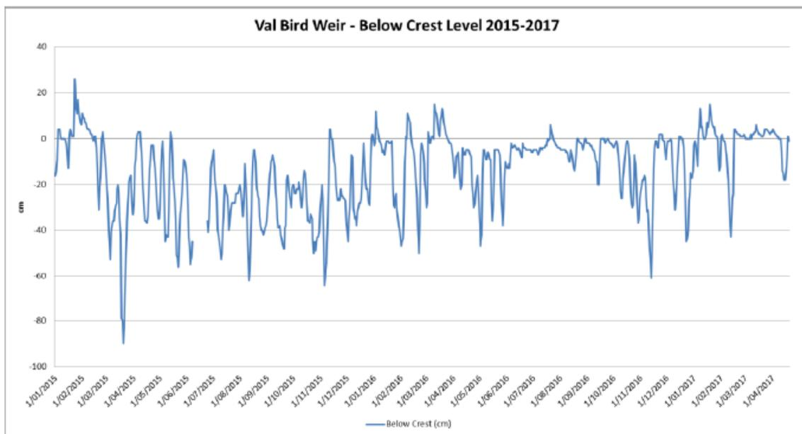
**Figure 4-3 – Val Bird Weir Water Levels (Kavanagh 2017)**
