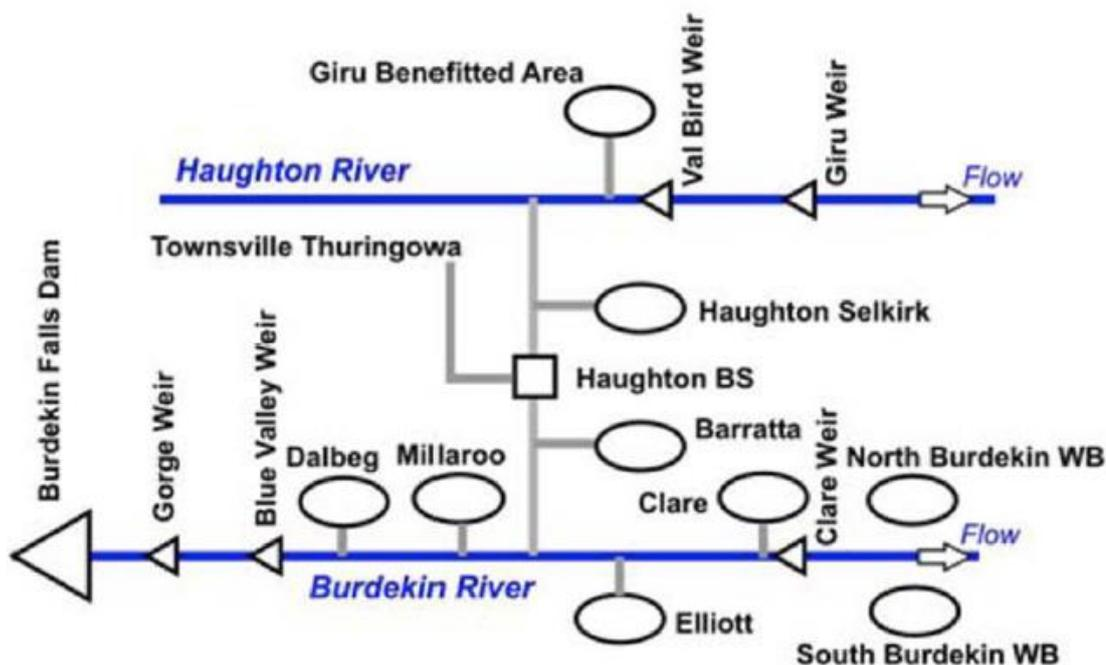
Figure 4-1 – Schematic of the BHWSS (OD Hydrology 2018)
