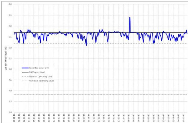
Figure 4 –Val Bird Weir water level behaviour
