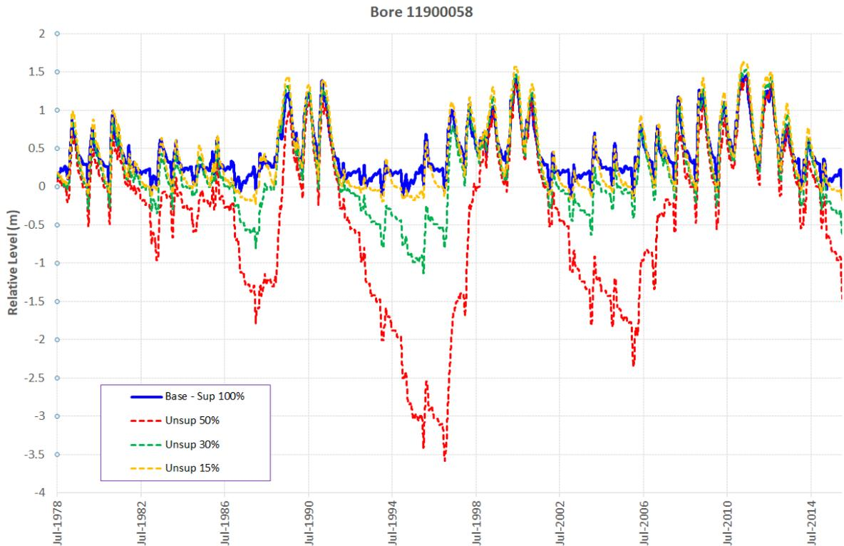
**Figure 4-4 – Modelled Aquifer Levels**
