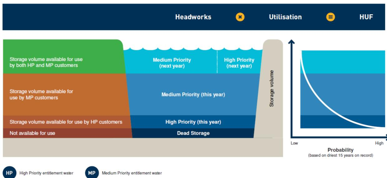
Figure 2-1 – How is the HUF Calculated? (SunWater 2018i)
