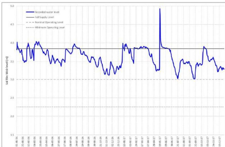
Figure 5 –Giru Weir water level behaviour
