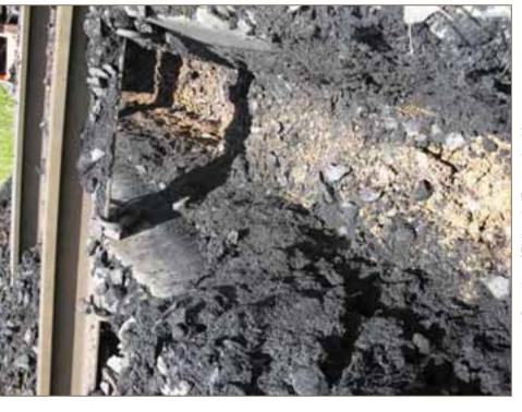
Sampling of Ballast by Destructive Means
