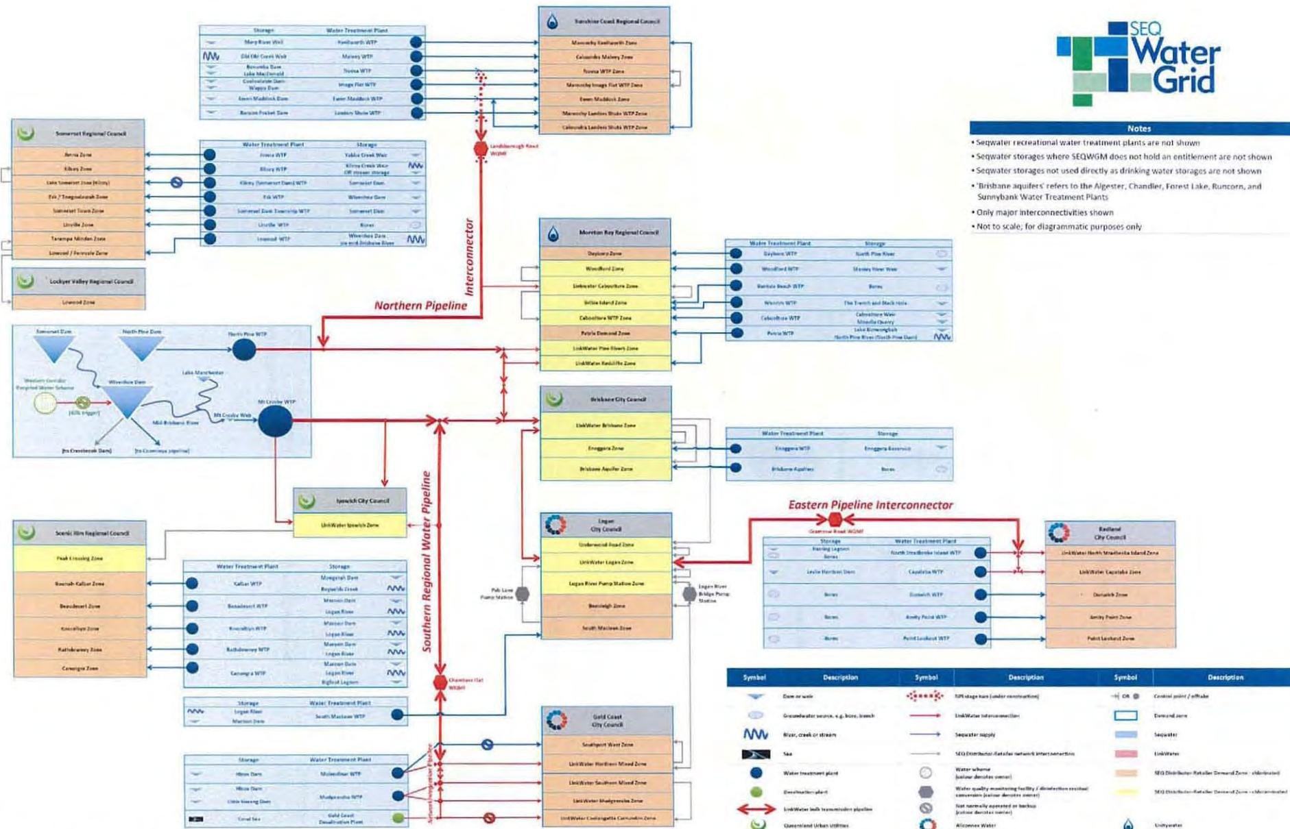
Figure 3: Water Grid supply zones and assets.
