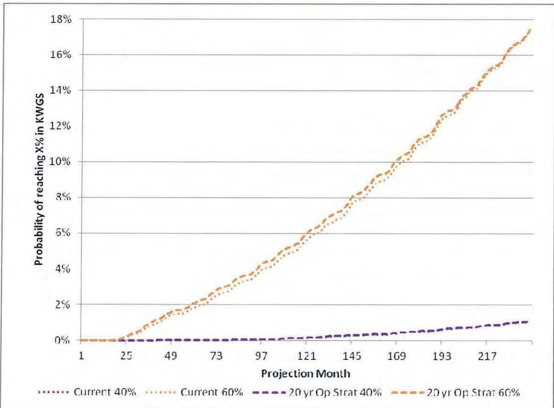
Figure 11: Probability of key Water Grid storages falling to 60% and 40% of combined capacity.
