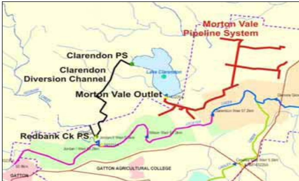
Figure 5.1: Morton Vale Pipeline Distribution System
