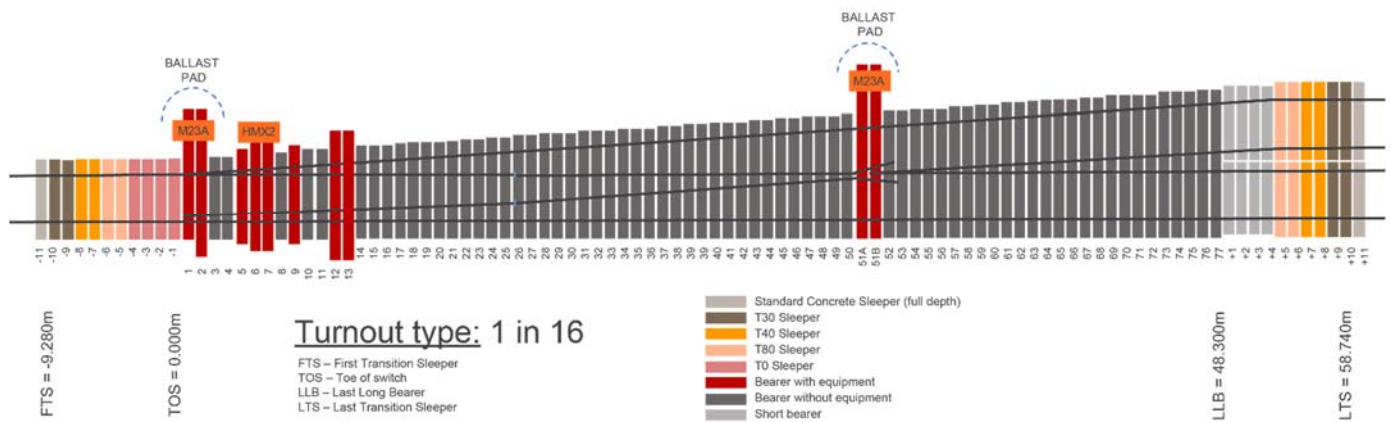
Figure 39 Turnout diagram: 1 in 16; 68.02m; represents 34% of total CQCN turnouts
