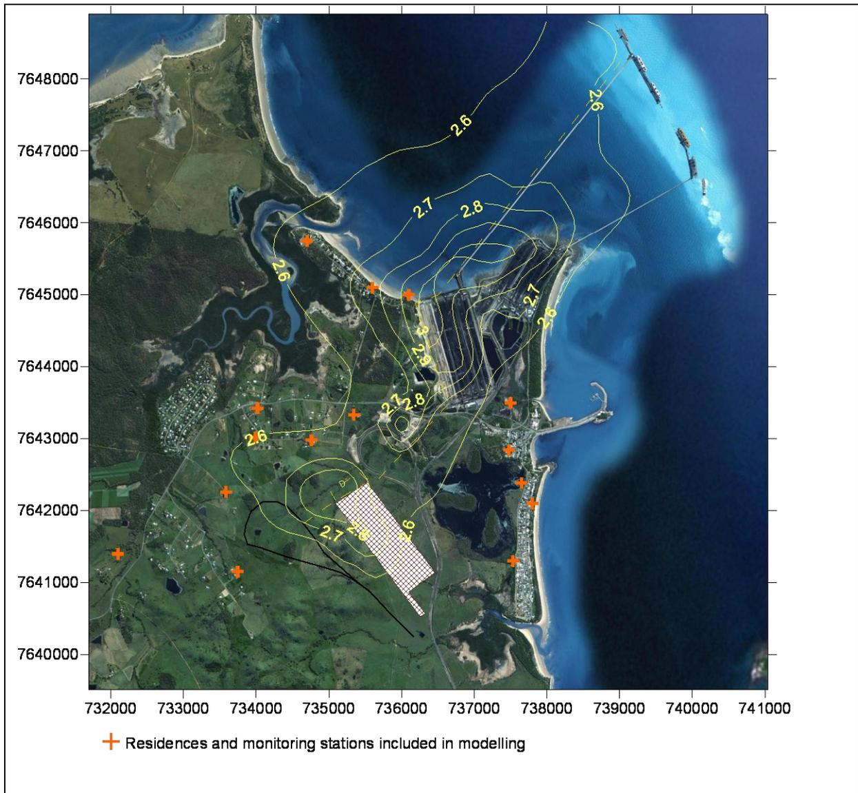
**Figure 7 Predicted annual average PM<sub>2.5</sub> ground-level concentrations for the Southern Stockyard Option with DBCT at 90 Mtpa, HPCT approved plus background levels**
