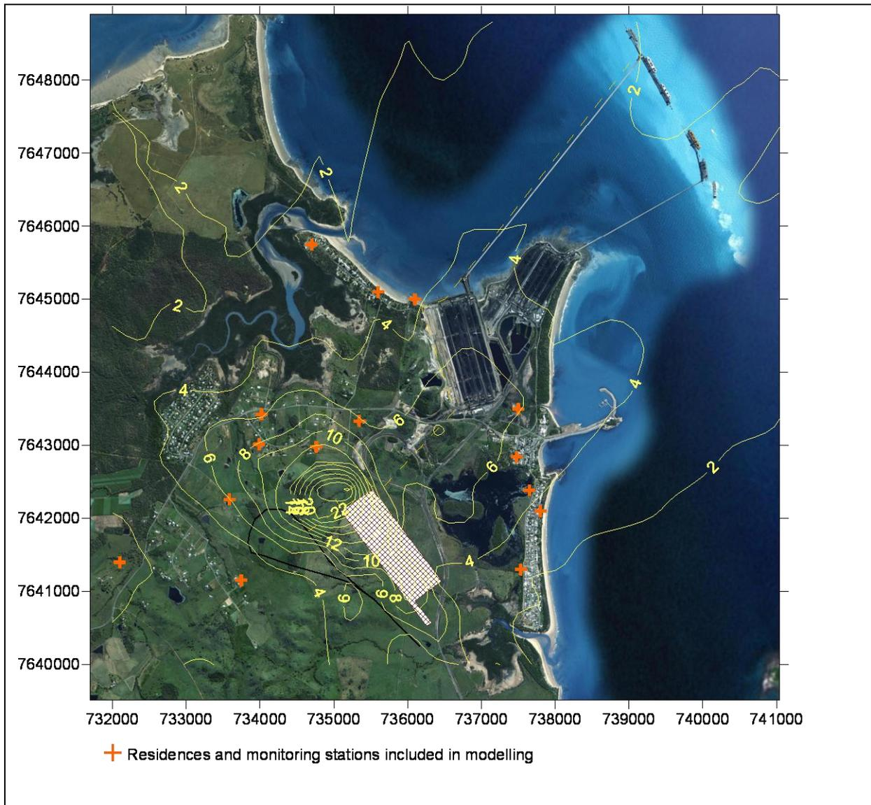
**Figure 8 Predicted 24-hour average PM<sub>10</sub> ground-level concentrations for the Southern Stockyard Option in isolation**
