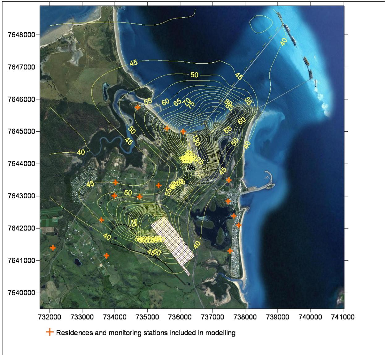
**Figure 13 Predicted annual average dust deposition rate for the Southern Stockyard Option with DBCT at 90 Mtpa, HPCT approved plus background levels**
