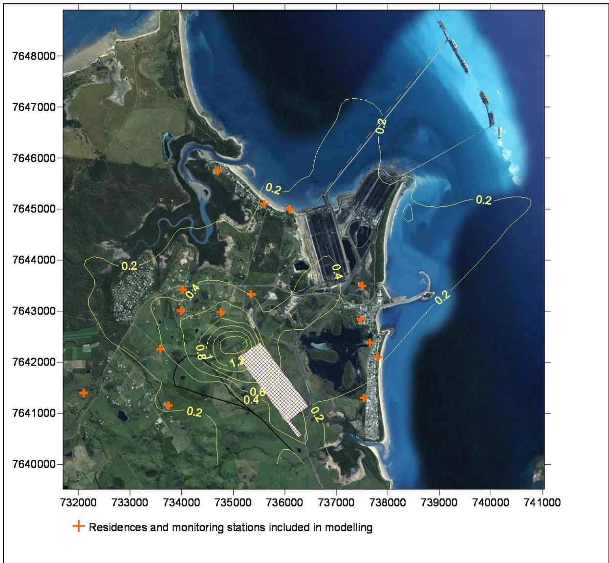
**Figure 4 Predicted 24-hour average PM<sub>2.5</sub> ground-level concentrations for the Southern Stockyard Option in isolation**
