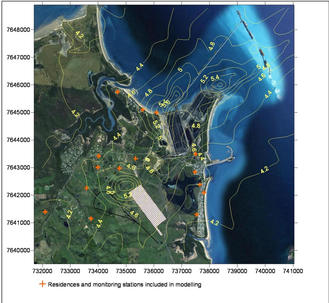
**Figure 5 Predicted 24-hour average PM<sub>2.5</sub> ground-level concentrations for the Southern Stockyard Option with DBCT at 90 Mtpa, HPCT approved plus background levels**
