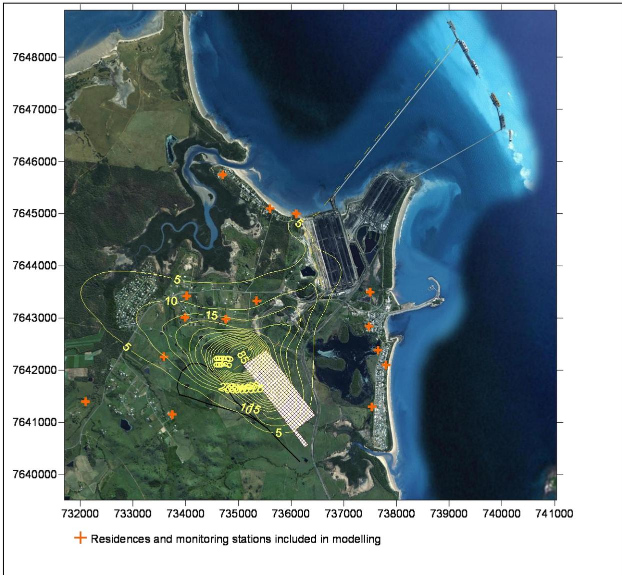
**Figure 12 Predicted annual average dust deposition rate for the Southern Stockyard Option in isolation**
