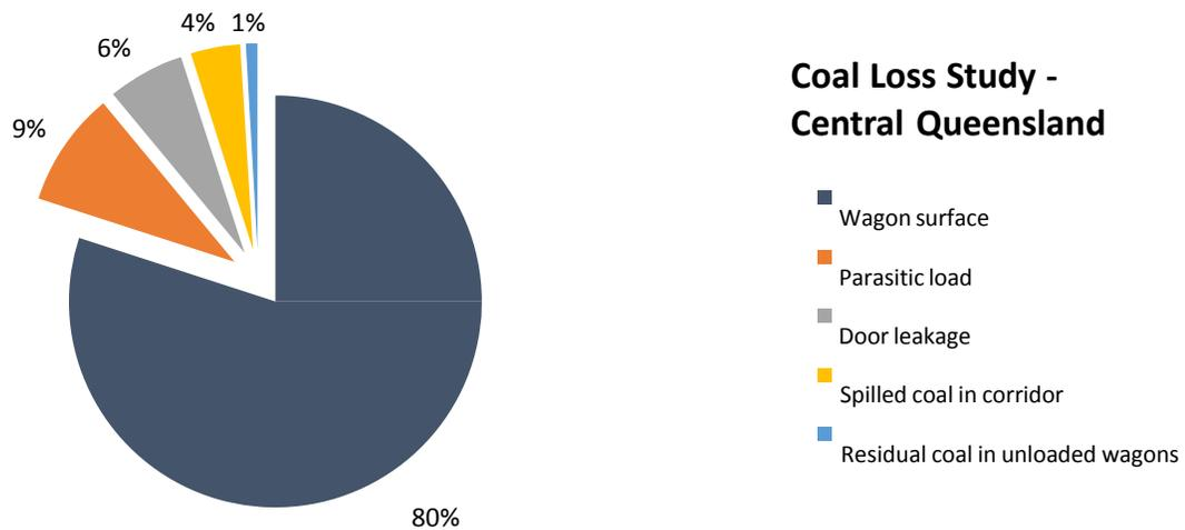
Figure 3. Sources of Coal loss
