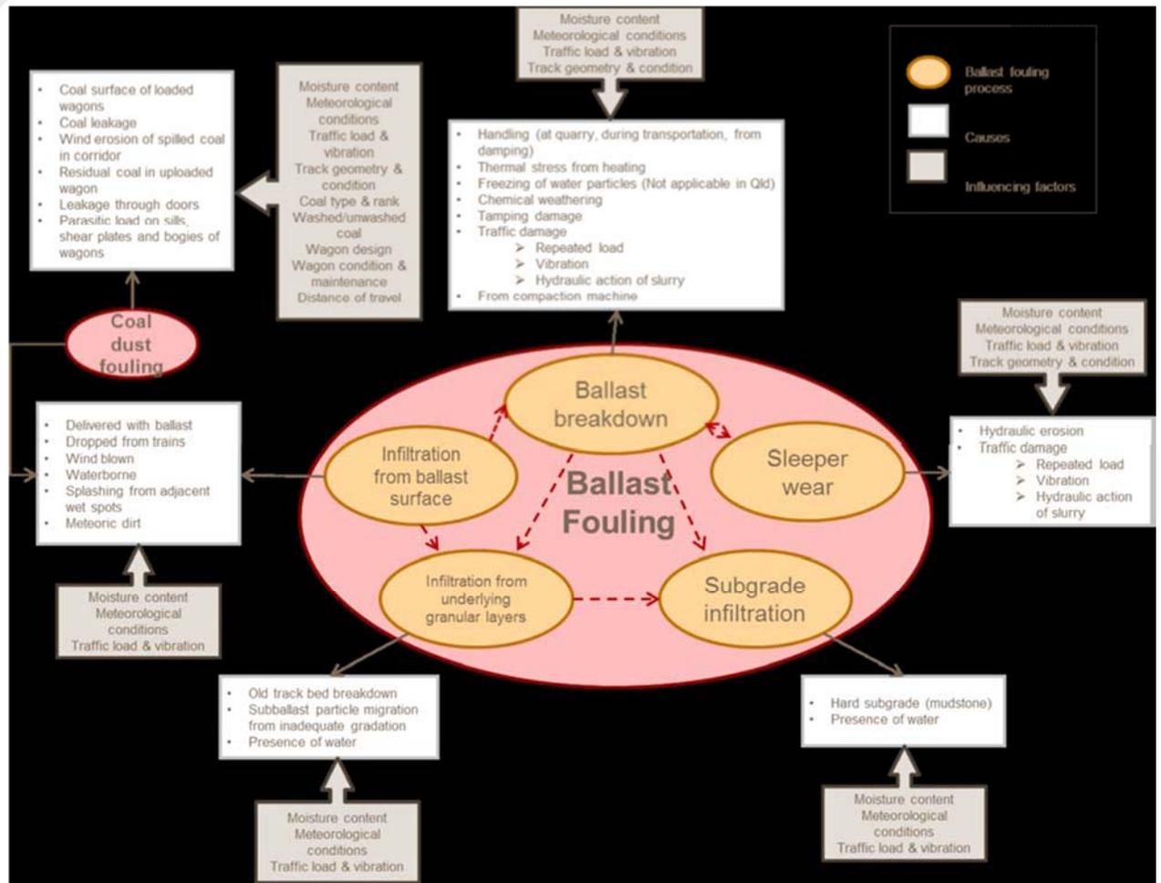
Figure 17. Ballast fouling inter-relationships
