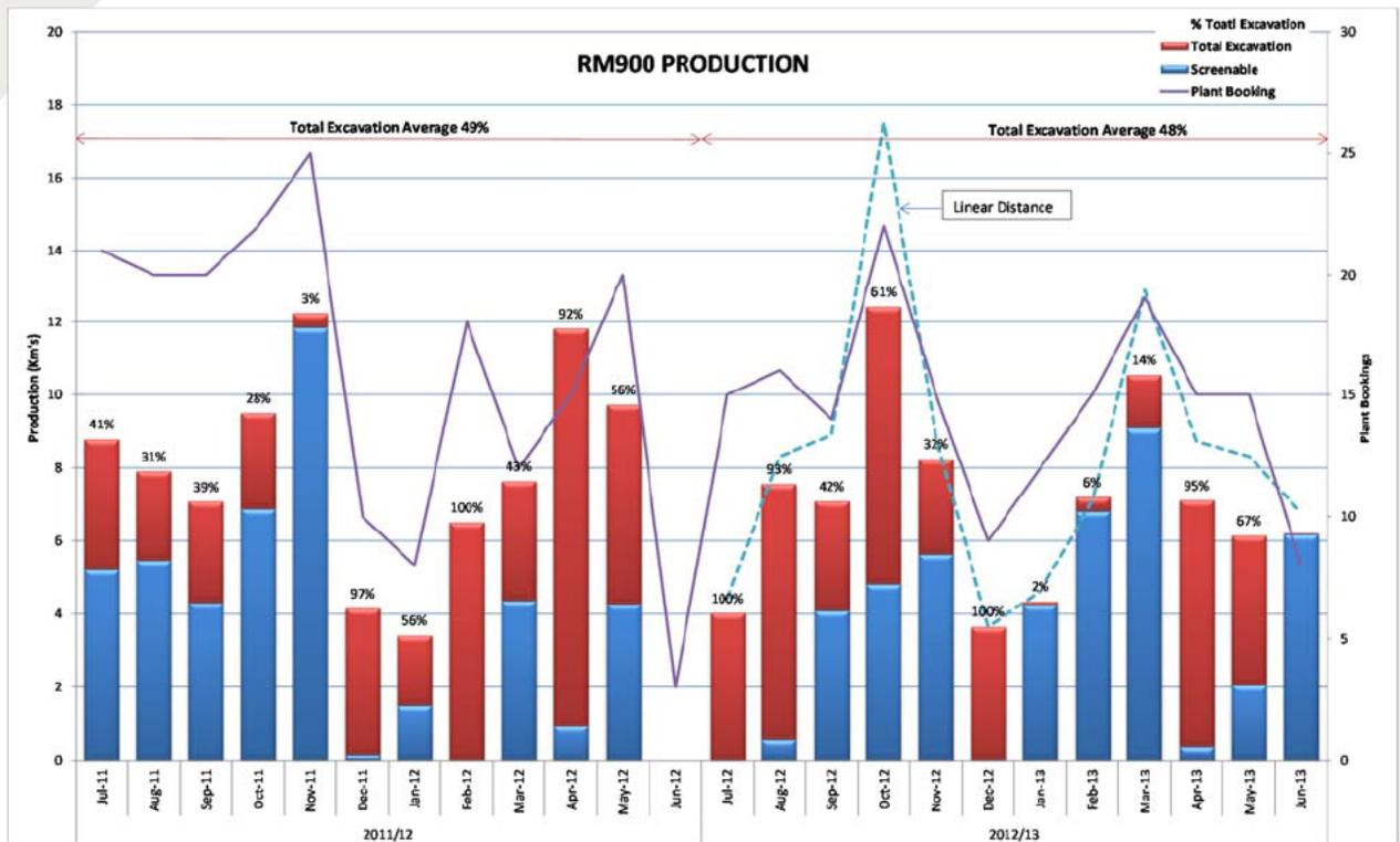
Figure 14. Ballast recycle rates for FY 2011/2012 and FY 2012/2013
