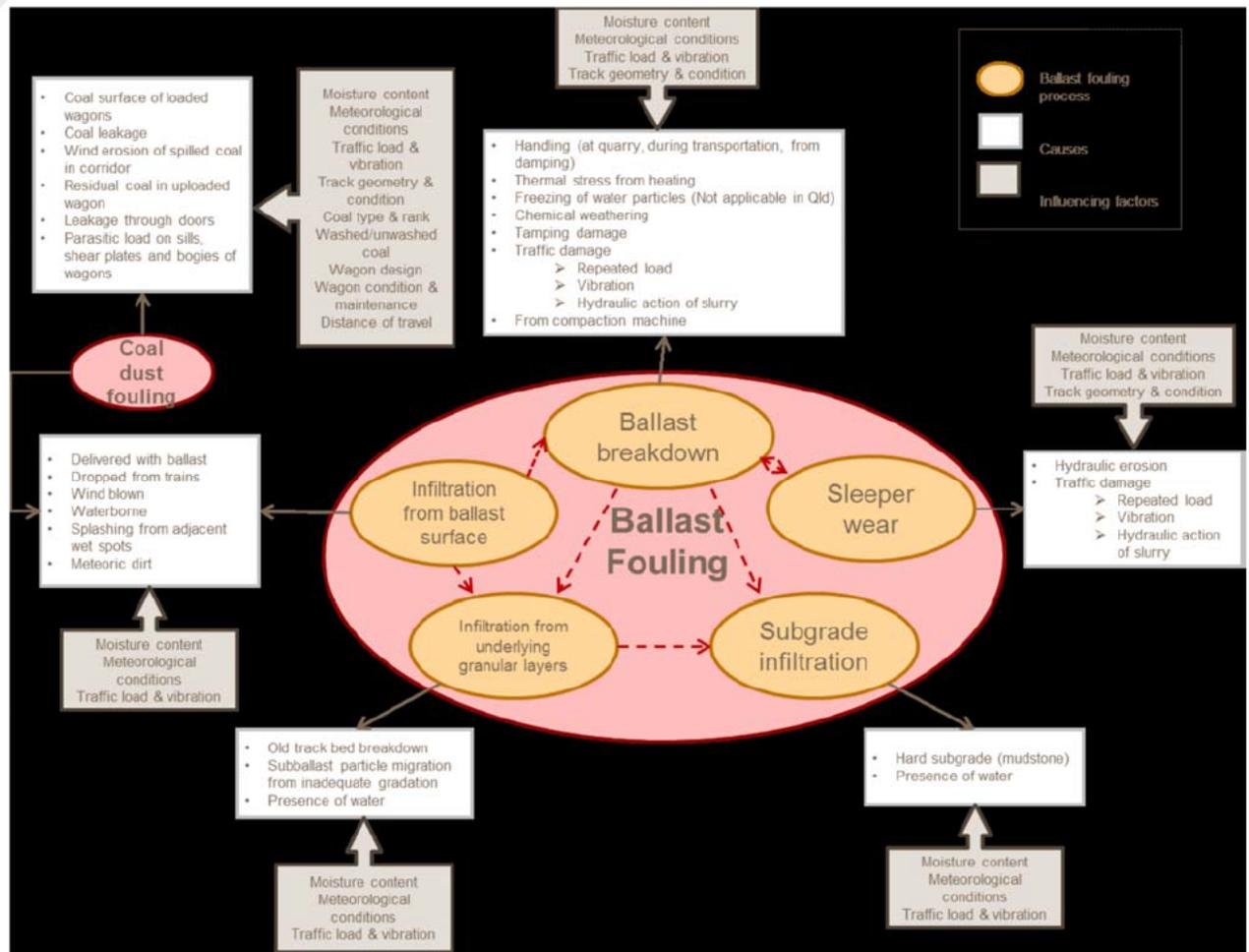
Figure 17. Ballast fouling inter-relationships
