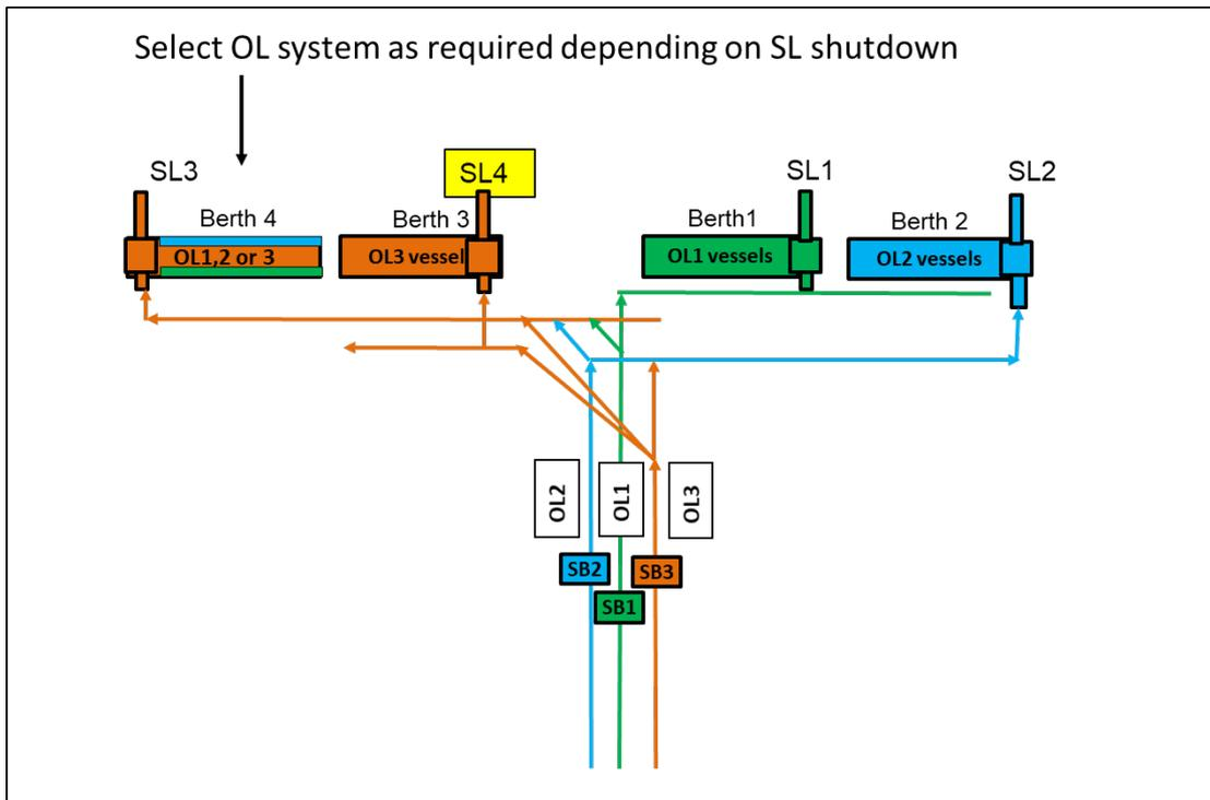
Figure 29- Proposed Outloading to Shiploader connectivity with SL4
