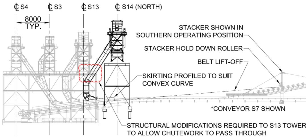
**Figure 35: Proposed alignment of IL4 conveyor S14 at the southern end of the yard**
