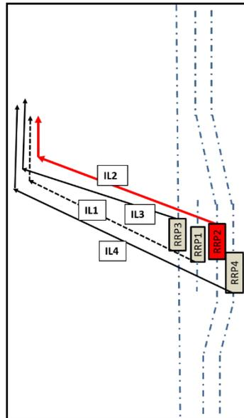
**Figure 34: IL system upgrade – Step 2 - Re-commission upgraded RRP2 and IL2, relocate RRP1 loop track to service RRP2, shutdown RRP1 and IL1. IL1 would likely remain shut-down until the future 9X expansion phase.**
