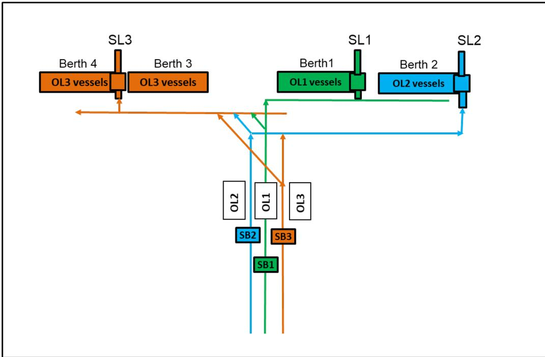
Figure 28- Existing Outloading to Shiploader connectivity
