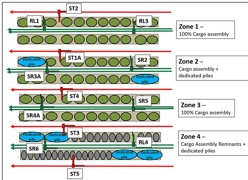
Figure 37: DBCT Stockyard following Zone 4 expansion
