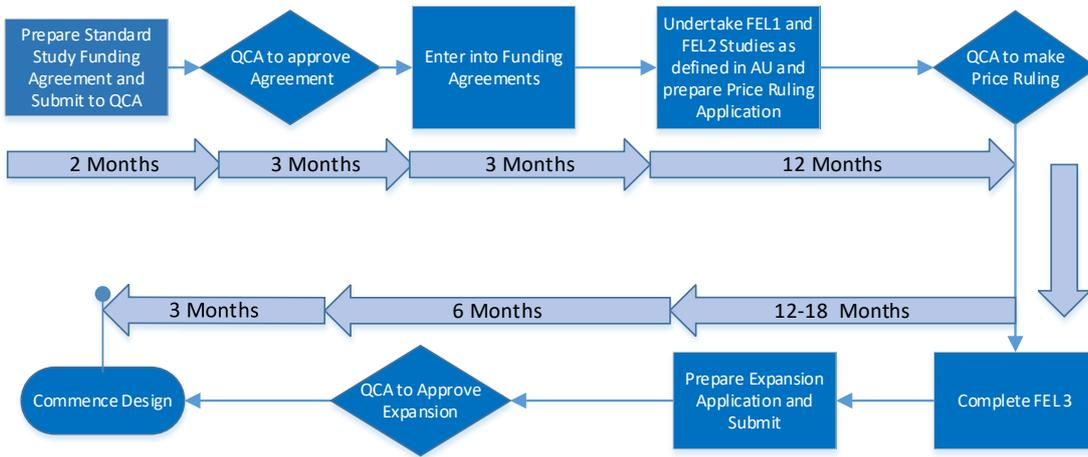
Figure 40: Expansion Approval process and indicative timeframes
