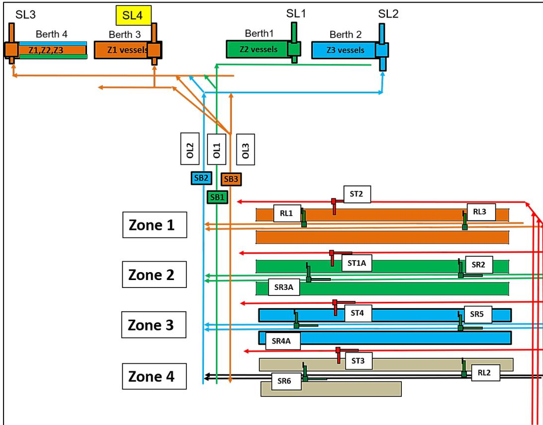
Figure 32: Proposed re-allocation of stockyard zones to OL systems following the SAP project
