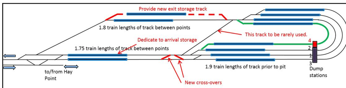
Figure 39: Proposed 8X rail loop modifications shown in red as proposed to be constructed with the IL4 dump station. The fourth rail loop in green would be constructed only at the later 9X stage.
