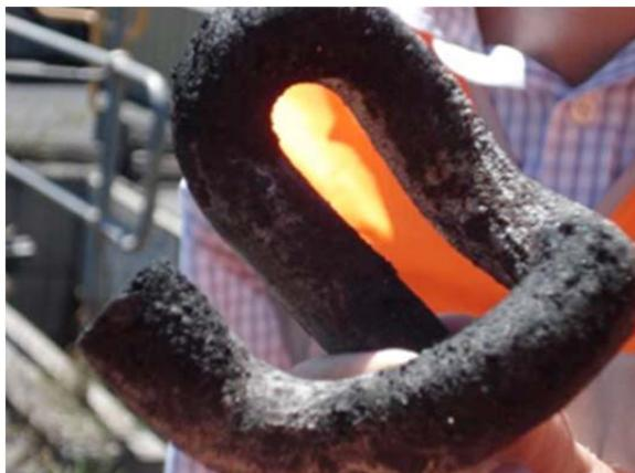
**Figure 6: Coal Corroded Fishplate**
