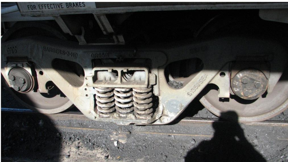
**Figure 4: Example of parasitic coal on a wagon**
