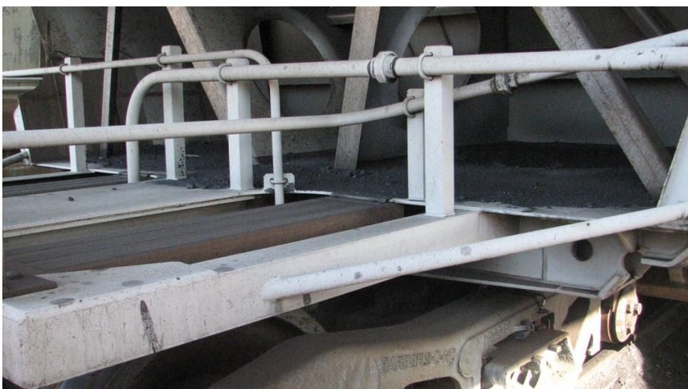
Carry back occurs when a wagon does not fully empty at an unloader station at a terminal. According to the survey conducted in 2007<sup>4</sup>, an average coal wagon was determined to have carry-back of approximately 0.36 tonnes; however the figure increased to 0.93 tonnes after torrential rains during the survey period.
