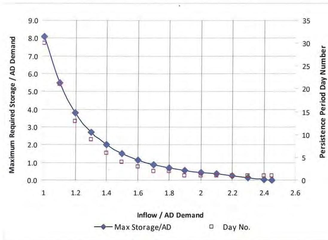
**Figure 5:** Example maximum persistence storage curve.
