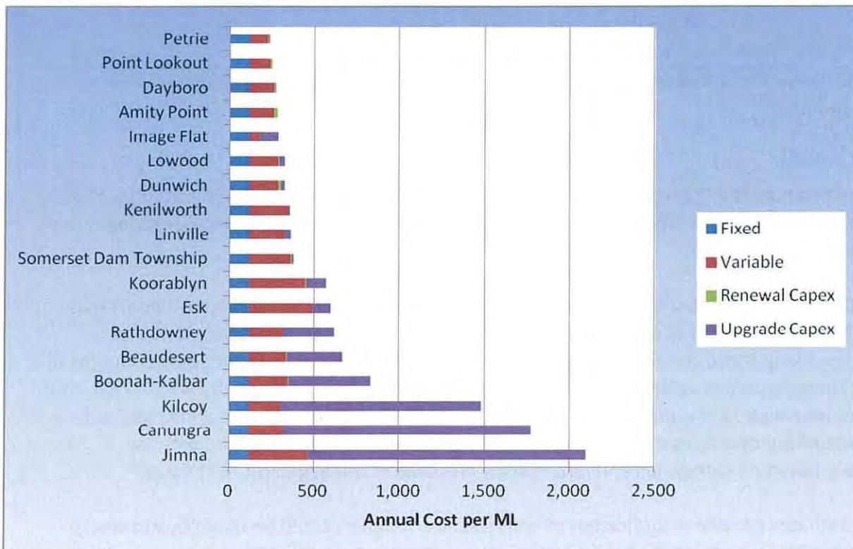
Figure 7: Annualised present value per ML capacity for stand-alone water treatment plants.
