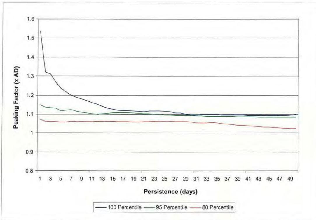
**Figure 4:** Typical persistence curves for varying probabilities of occurrence.
