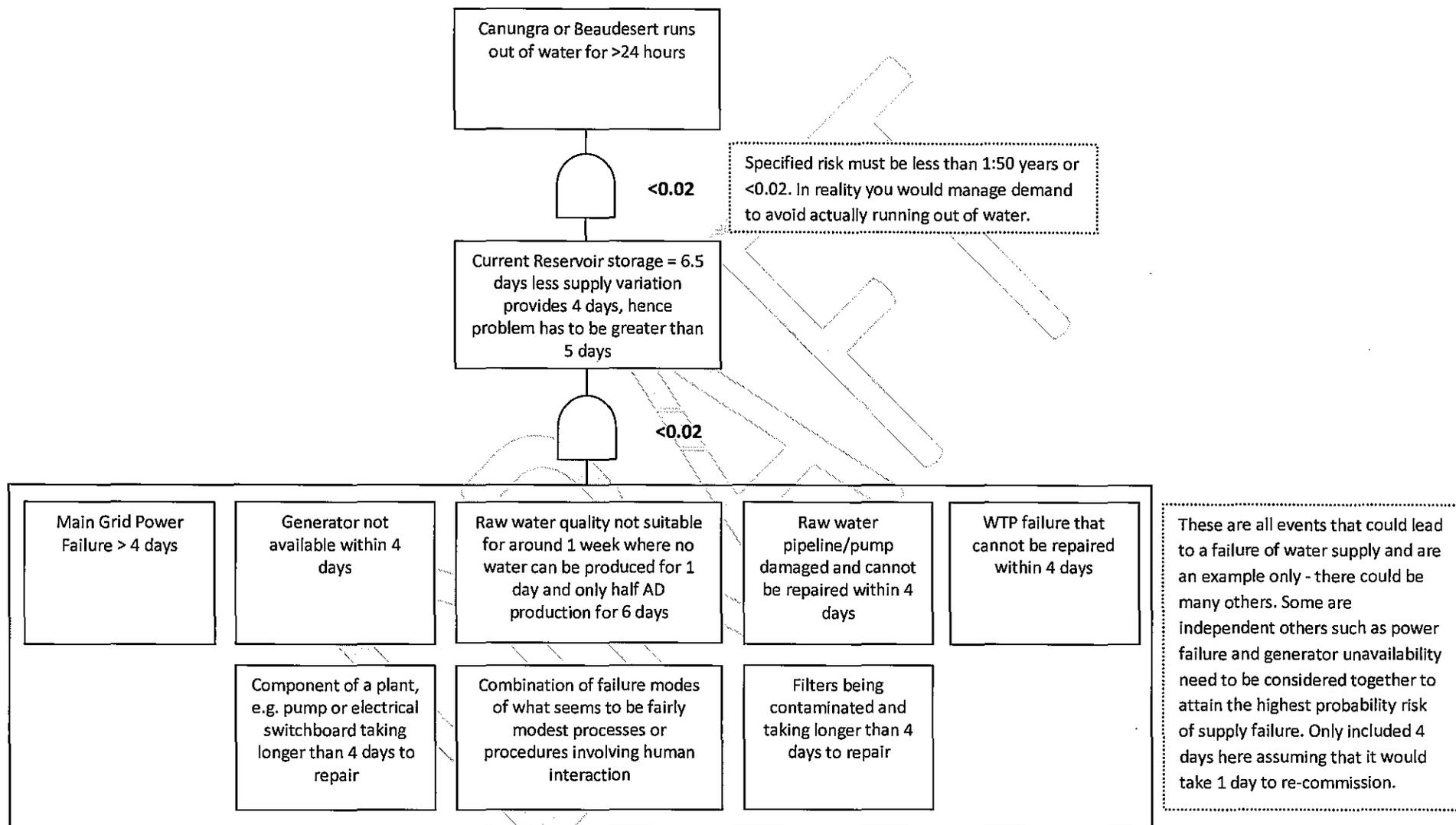
Figure 6: Key risks to be considered as part of Failure Modes, Effects and Criticality Assessment.
