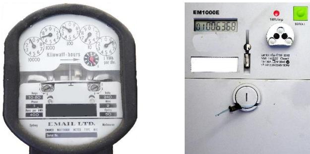
Advanced digital meters (smart meters), record electricity usage, and in some cases demand, every 30 minutes. They also have communication capability allowing meters to be read remotely, as well as to be reconfigured, disconnected and reconnected remotely.
