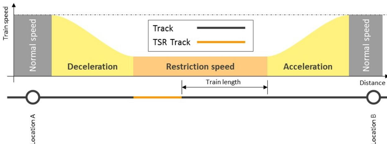
**Figure 14: Assumed impact to train speed used to calculate TSR impact to SRT**
