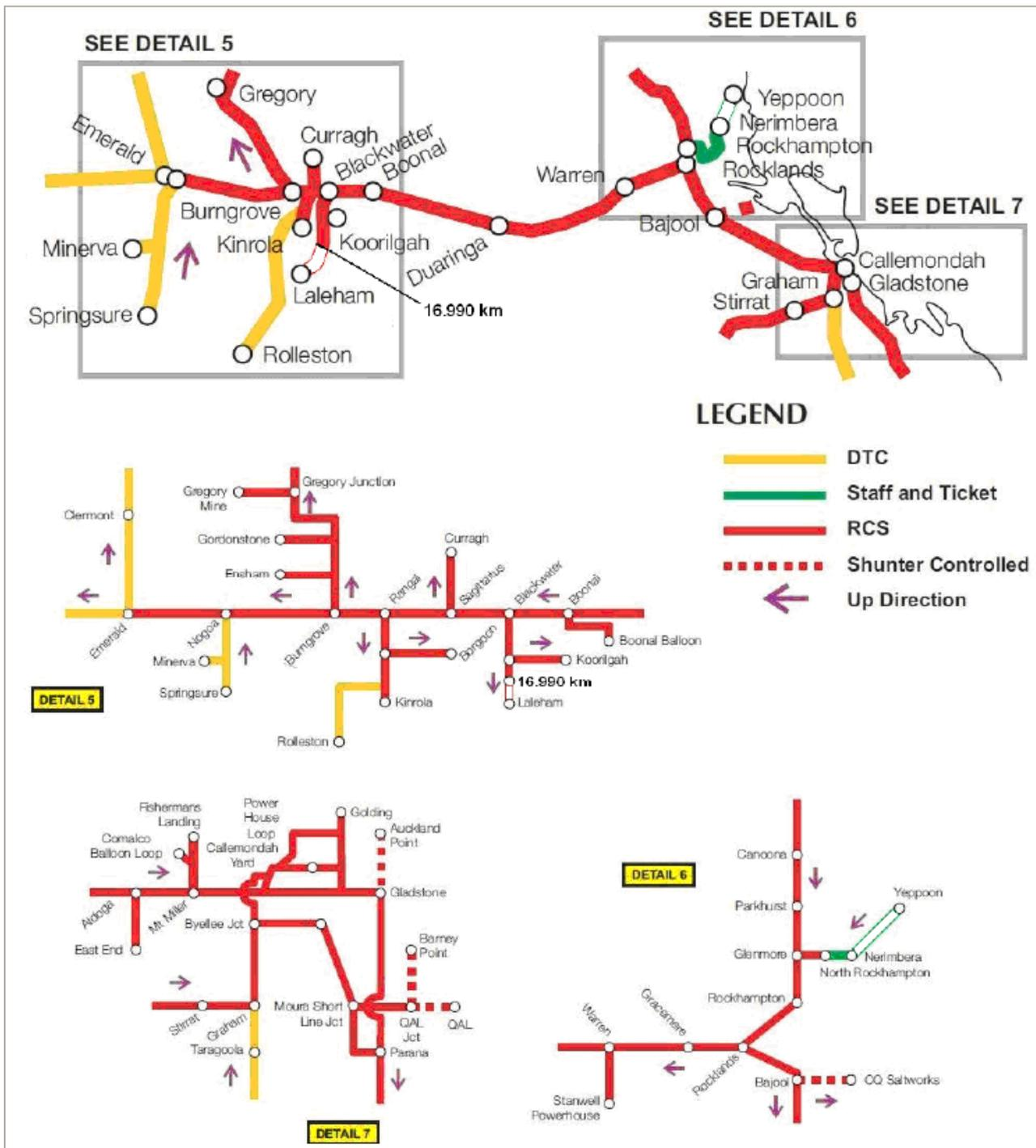
Figure 6: Blackwater system train control map
