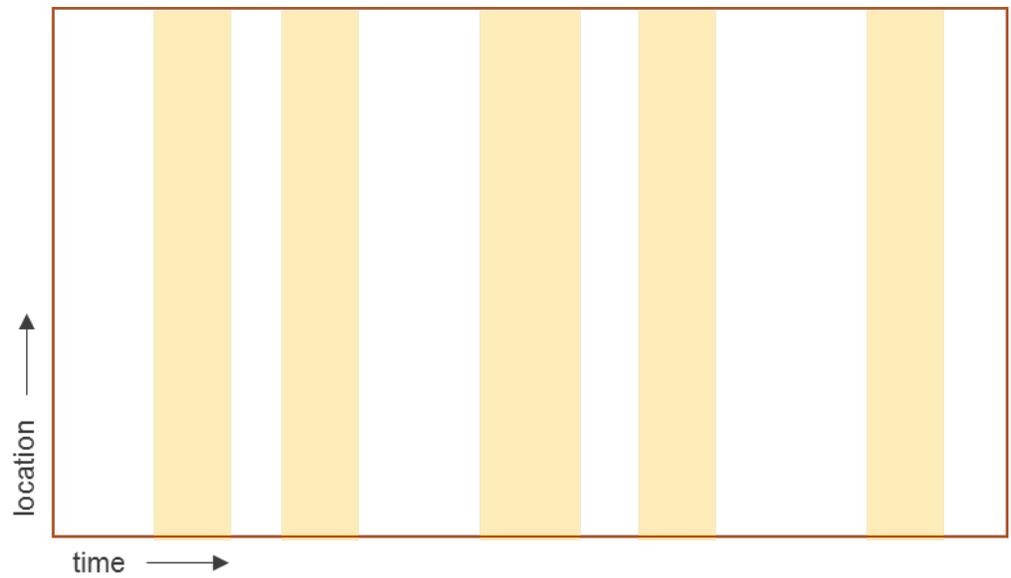
PACE generates a series of possessions (VPP) to replicate the scope of work taking into account resource constraints and production rates.
