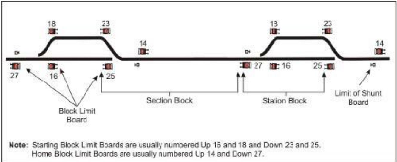
Figure 8: DTC Blocks and Position of Block Limit Boards
