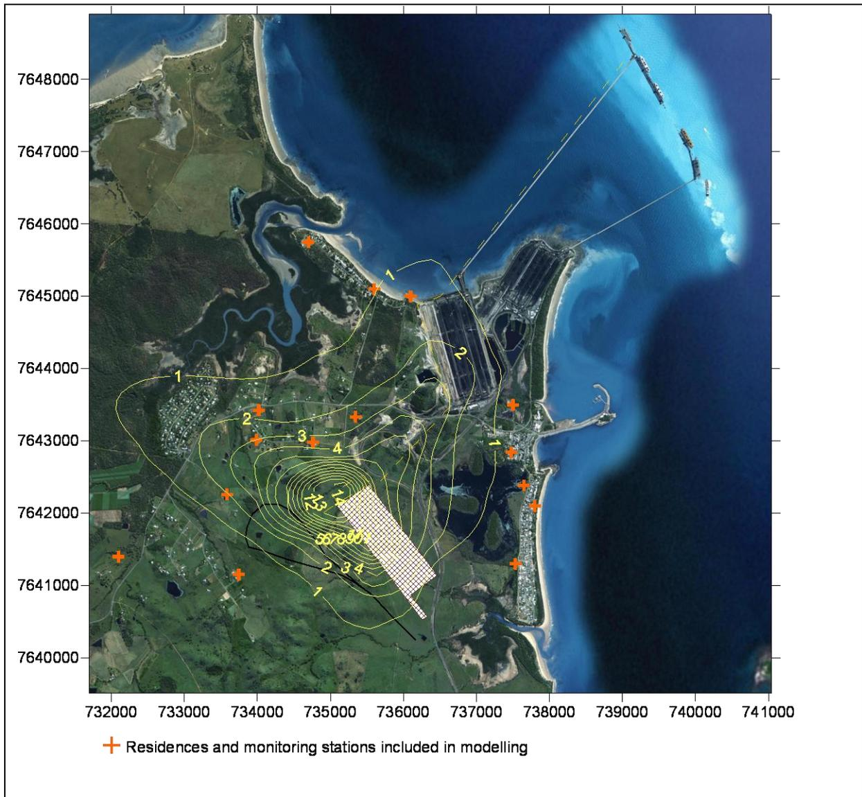
**Figure 10 Predicted annual average TSP ground-level concentrations for the Southern Stockyard Option in isolation**
