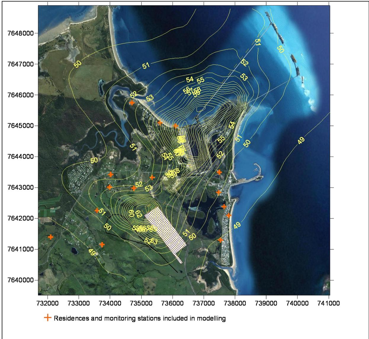
**Figure 11 Predicted annual average TSP ground-level concentrations for the Southern Stockyard Option with DBCT at 90 Mtpa, HPCT approved plus background levels**
