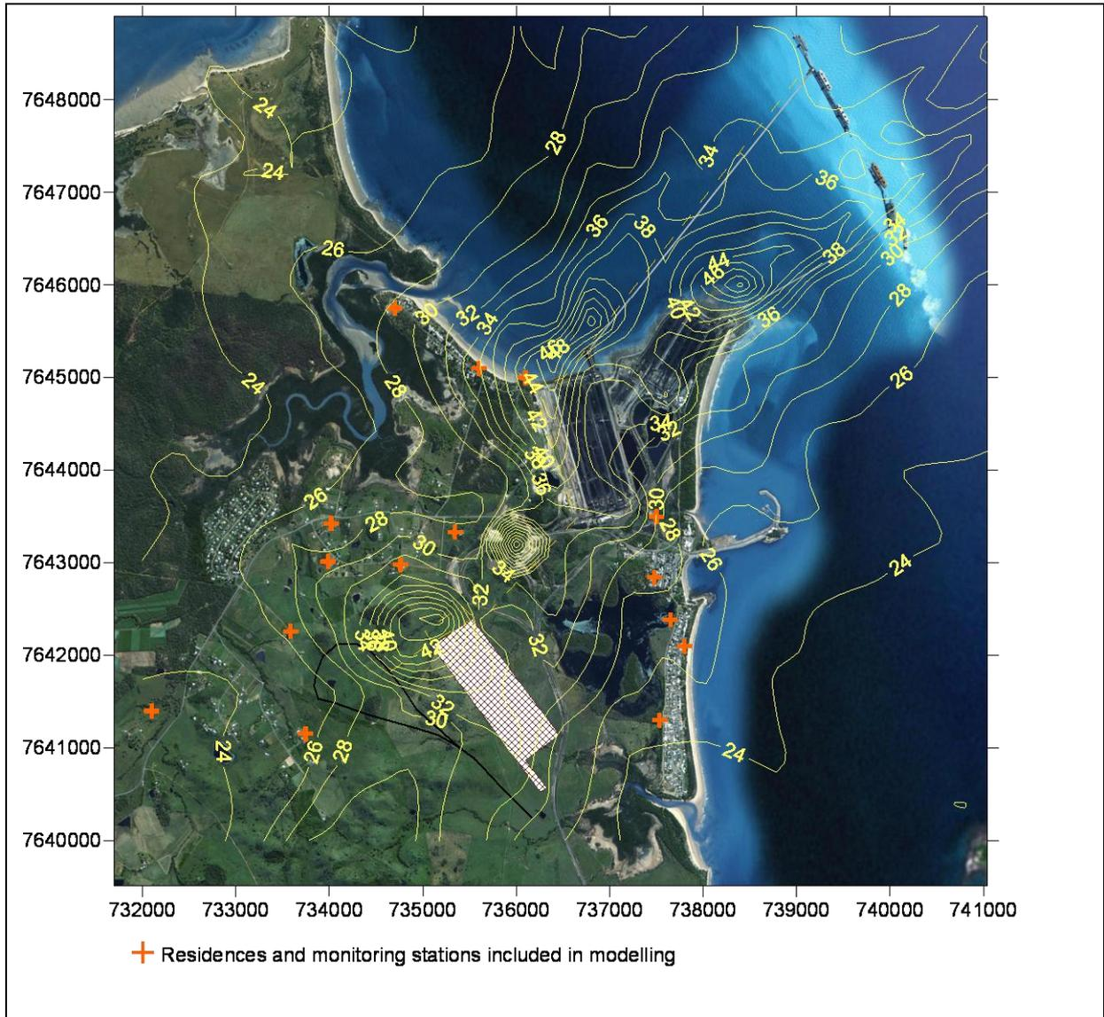
**Figure 9 Predicted 24-hour average PM<sub>10</sub> ground-level concentrations for the Southern Stockyard Option with DBCT at 90 Mtpa, HPCT approved plus background levels**
