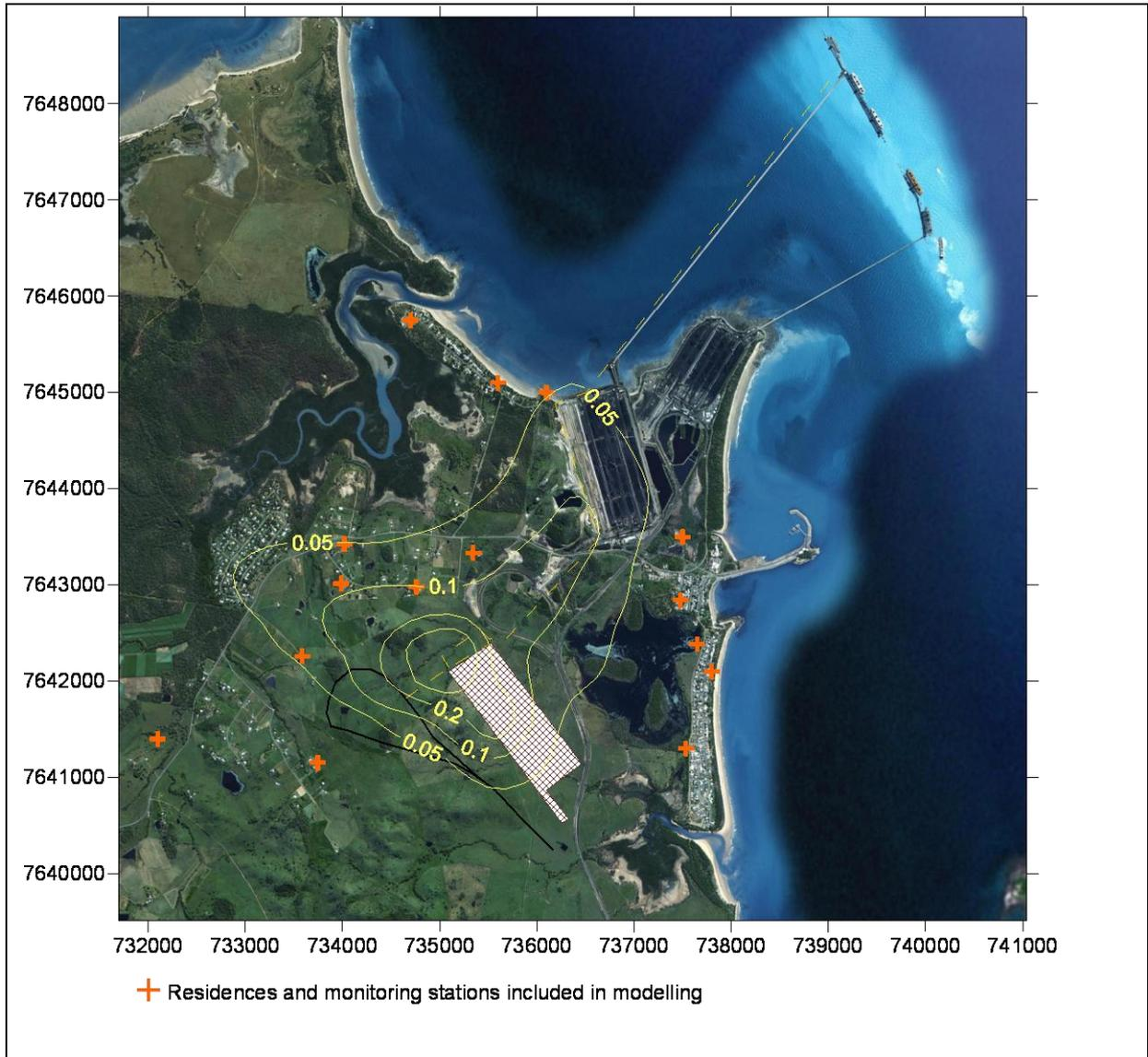
**Figure 6 Predicted annual average PM<sub>2.5</sub> ground-level concentrations for the Southern Stockyard Option in isolation**
