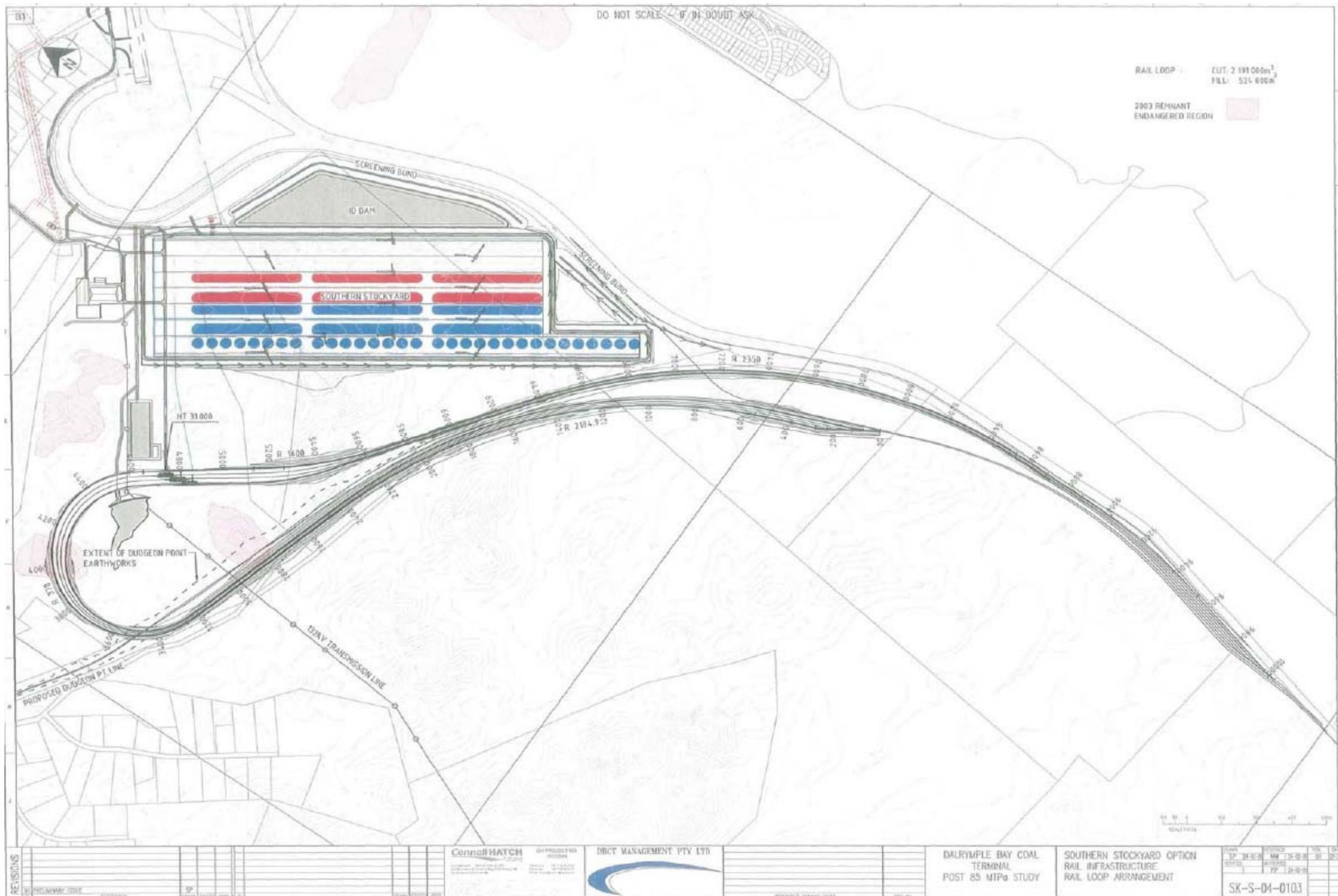
Figure 24 – DBCT 9X expansion Southern Stockyard – rail loop/inloading and stockyard configuration
