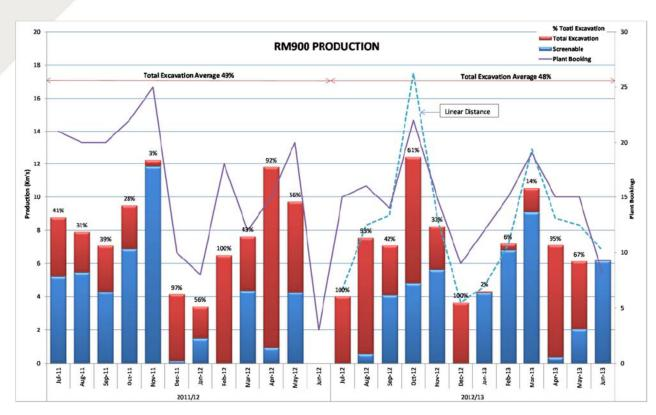
Figure 14. Ballast recycle rates for FY 2011/2012 and FY 2012/2013
